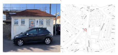
Former single storey public toilet of circa 200 sqft with concrete tiled pitched roof, rough cast rendered elevations constructed in the late 1930's with male and female sides. It has been closed for many years and is in poor condition and subject to vandalism.
